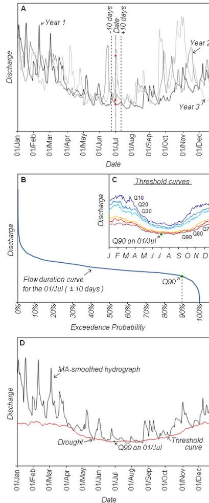
**Fig. 2.** Calculation steps from annual discharge series to a daily threshold curve.
