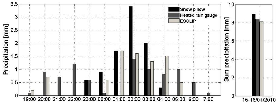
**Fig. 6.** Comparison of precipitation measured with snow pillow, with a heated rain gauge and ESOLIP for a single mixed snow and rainfall precipitation event ( $T_w$  decreasing from 4 to  $-2.5\text{ }^\circ\text{C}$ ) at the test site in Stubai: left hourly values, right total sum (15 May 2012).
