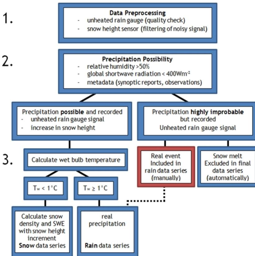
**Fig. 1.** Scheme of the proposed methodology to estimate solid and liquid precipitation (ES-OLIP).
