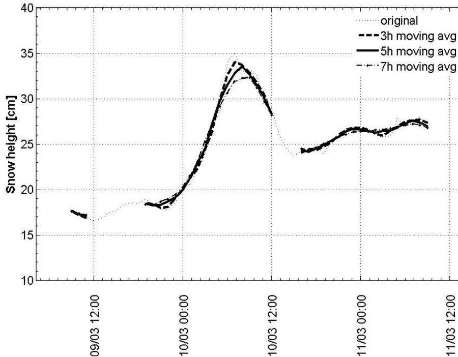
**Fig. 2.** Comparison of different moving average (avg) intervals for snowfall events to reduce the noise in the snow height signal for a period with snowfall at the Matsch test site (see also Table 2).
