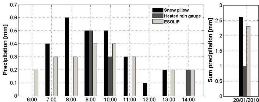
**Fig. 5.** Comparison of precipitation measured with a snow pillow, a heated rain gauge and ESOLIP for a single snowfall event ( $T_w -5^\circ\text{C}$ ) at the test site in Stubai: hourly values on the left, daily sum (28 January 2010) on the right.
