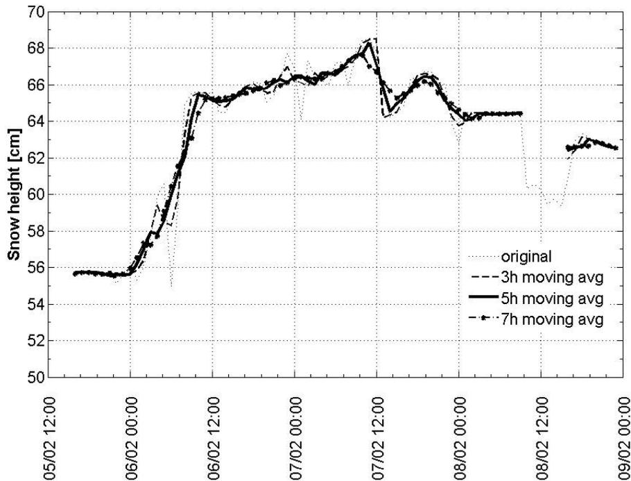
**Fig. 3.** Comparison of different moving average (avg) intervals to reduce the noise in the snow height signal for a snowfall period followed by sunny weather at the Stubai test site. The moving averages were applied only if weather conditions allowed snowfall (see also Table 2).
