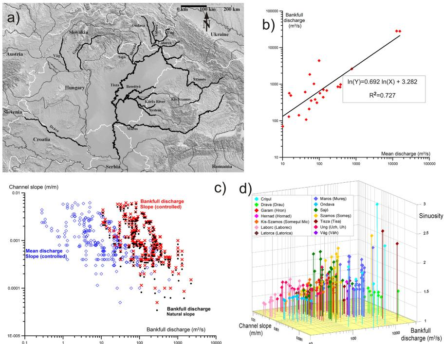
**Figure 1.** Corrections and points. **(a)** The water discharge, slope and sinuosity values of the displayed rivers (black) of the Pannonian Basin were used for this study; **(b)** the mean and bankfull discharges of van den Berg (1995), and the fitted line; **(c)** the result of the corrections; **(d)** the abstract surface was fitted onto these points (see black points on **c**). The different colours mean different rivers.
