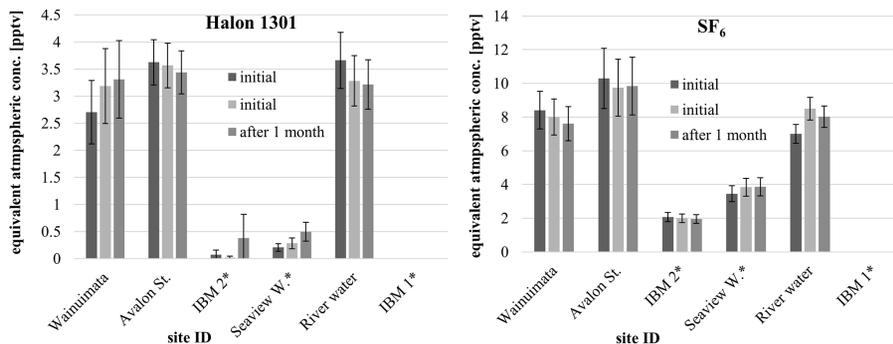
**Figure 9.** Comparison of Halon-1301 concentration in 1 L water samples analysed directly after sampling (2 of 3) and after 7 weeks storage (1.2 years for Hutt River water sample) at 14 °C (1 of 3). \* Anoxic water samples.
