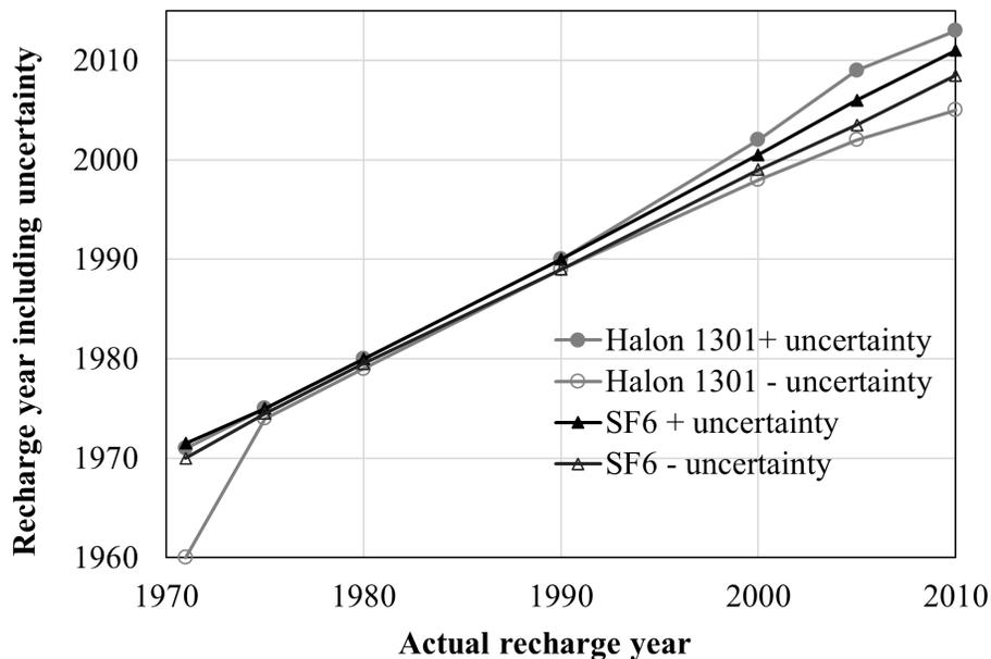
**Figure 5.** Effect of relative analytical uncertainty on inferred piston flow recharge year for SF<sub>6</sub> and Halon-1301.
