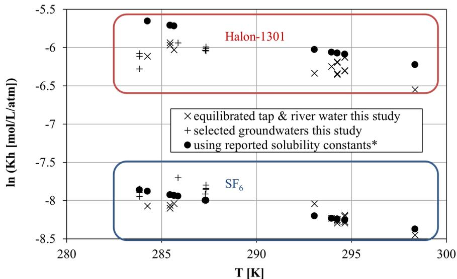
**Figure 6.** Estimated solubility of Halon-1301 and SF<sub>6</sub> in equilibrated tap water, river water, and aerobic young groundwater in comparison to reported solubility data. \* Data from Deeds (2008) for Halon-1301 and Bullister et al. (2012) for SF<sub>6</sub>.
