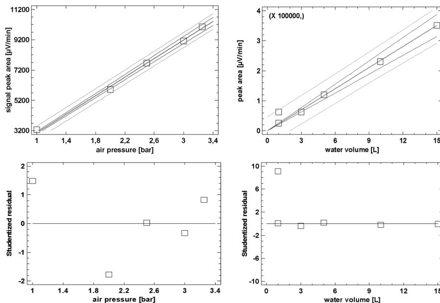
**Figure 4.** Assessment of linearity of the ECD signal towards Halon-1301 using 10 mL modern air at different pressures (left) and water at different volumes (right) showing an almost linear signal to pressure/volume (upper) and acceptable residuals (lower), lines in upper graphs represent the best least square fit, fit with SD of slope and 95 % confidence interval.
