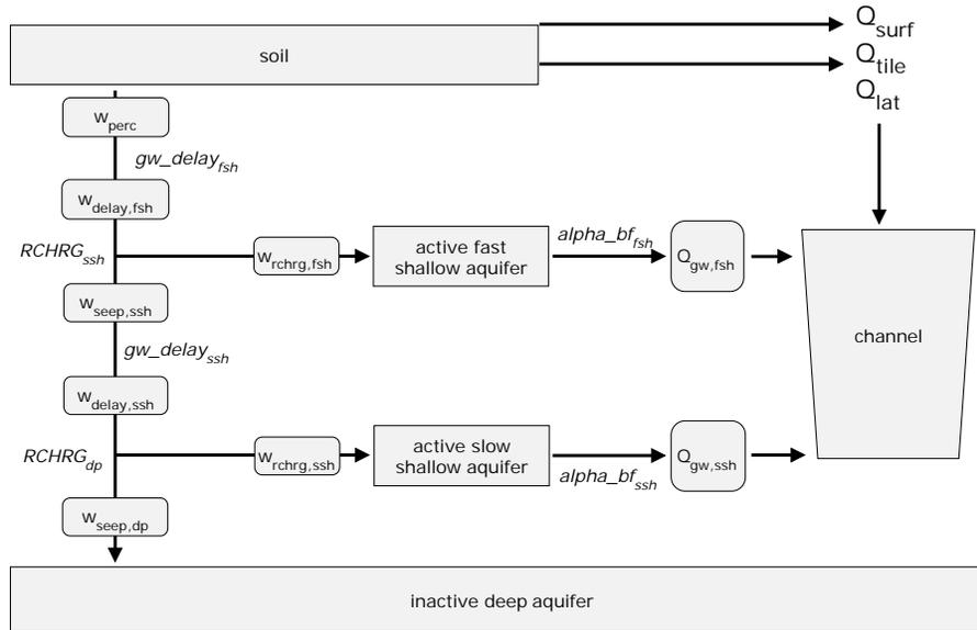
**Figure 2.** Description of the main groundwater processes and its parameters (highlighted in italic) of SWAT<sub>3S</sub> (cf. Pfannerstill et al., 2014a).
