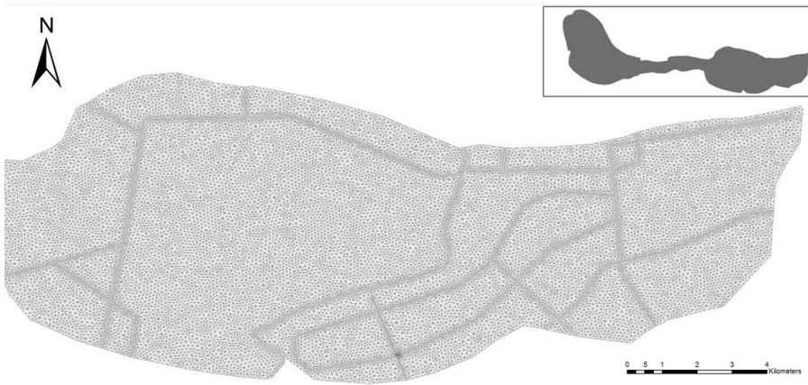
**Figure 4.** The 2-D hydraulic model mesh of Gongshuangcha Polder and its regional enlarged view.
