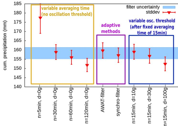
**Figure 9.** The values for cumulative precipitation together with the SD regarding the measurements of the 18 different lysimeters for different parameter selections and the two adaptive methods.
