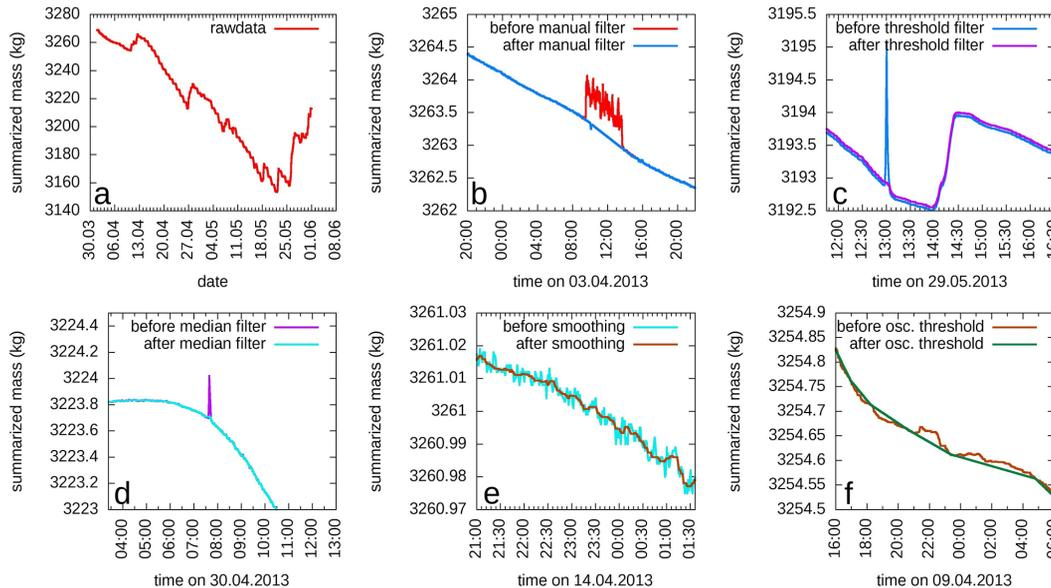
**Figure 3.** Examples for the effect of the different filtering steps on the mass data (here: summarized mass of lysimeter and seepage water tank of lysimeter BL1-L1). Please note the different scaling of the y axes. **(a)** raw data, **(b)** manual filter, **(c)** threshold filter, **(d)** median filter, **(e)** smoothing filter, **(f)** oscillation threshold filter.
