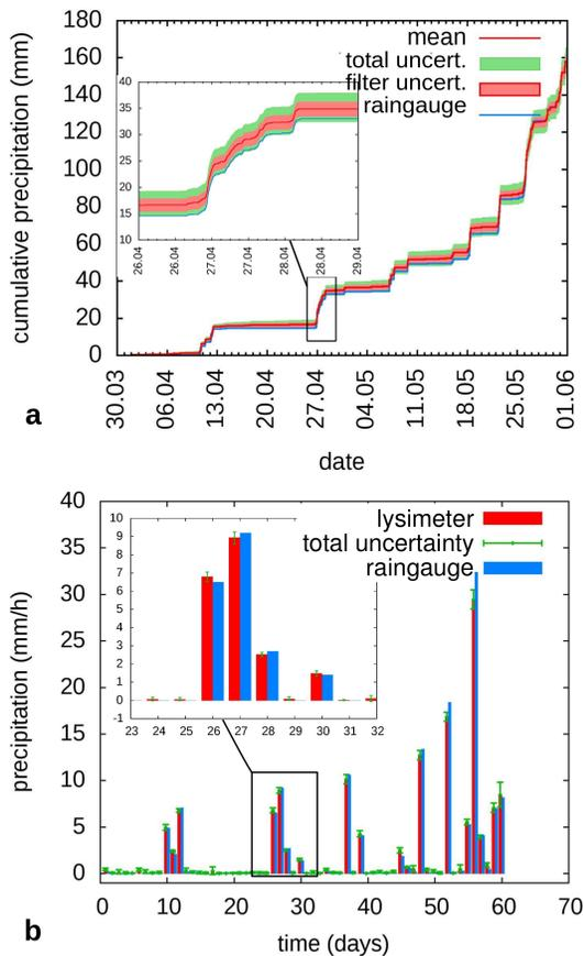
**Figure 8.** The calculated precipitation with its uncertainties as cumulative precipitation **(a)** and daily precipitation **(b)**. The total uncertainty is the sum of the estimated filtering uncertainty and the SD of the different measurements on the 18 lysimeters.
