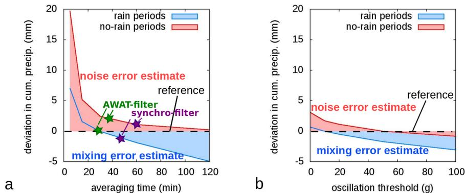
**Figure 11.** Effects of averaging time **(a)** and oscillation threshold value **(b)** on the estimates for the mixing error and the noise error. The error estimates of the AWAT-filter and the synchro-filter are indicated in **(a)** with green stars for the AWAT-filter and purple stars for the synchro-filter.
