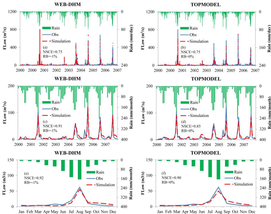
**Figure 3.** Observed and simulated flow using WEB-DHM and TOPMODEL from 2000 to 2007.
