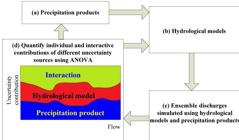
**Figure 4.** Diagrammatic flowchart of the proposed framework for quantification of uncertainty contributions to ensemble discharges simulated using precipitation products.
