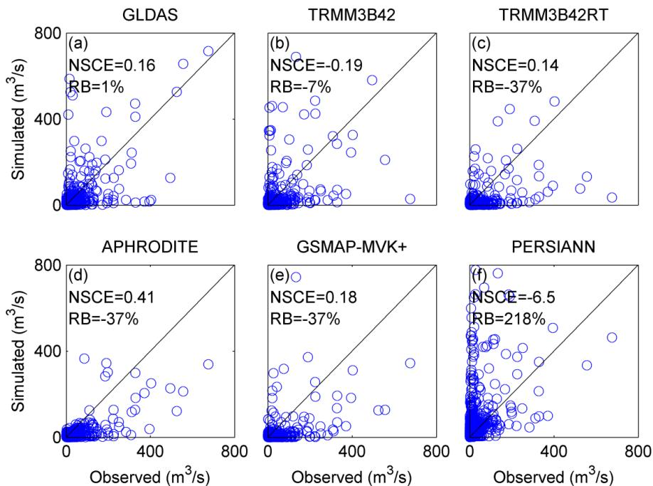
**Figure 12.** Scatterplots of simulated discharges with WEB-DHM against observations at a daily scale.
