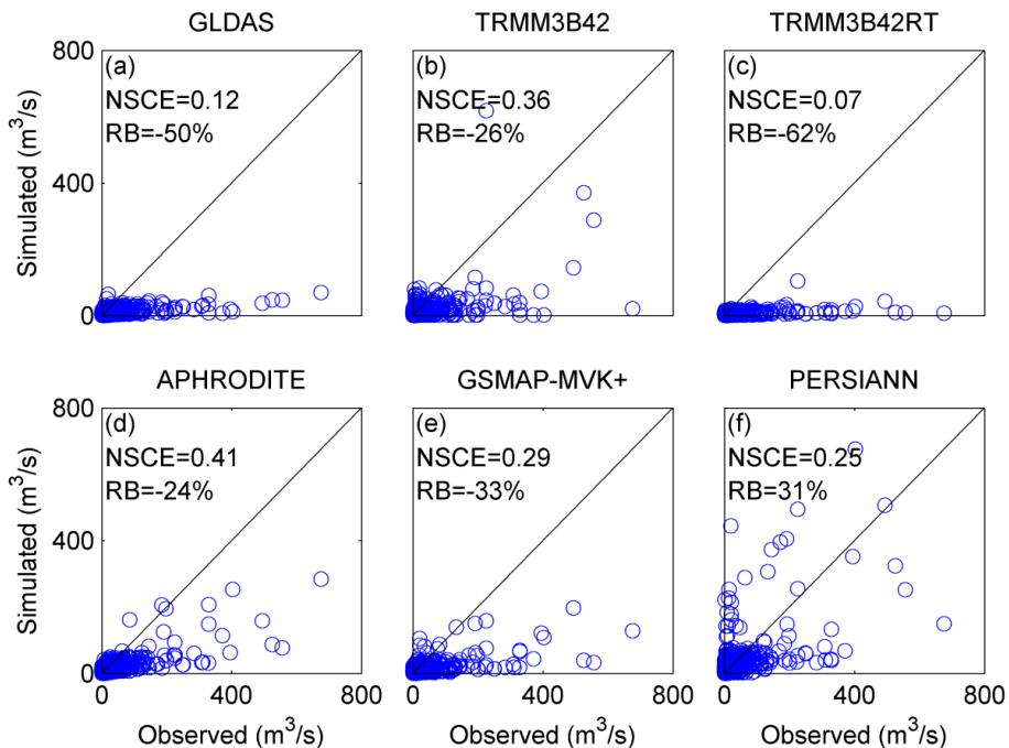
**Figure 13.** Scatterplots of simulated discharges with TOPMODEL against observations at a daily scale.
