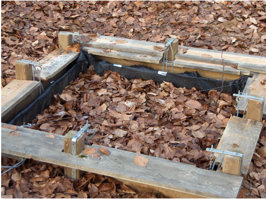
Fig. 3. Interception device in the Huewelerbach catchment on January 2006. The upper basin is filled with leave litter.
