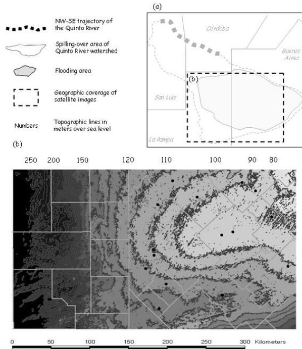
**Fig. 2.** (a) graphic of Fig. 1 showing the area of the Quinto river watershed, (b) Topographic features of the flooding area from Landsat images showing the strip that separates highlands from lowlands on 110–120 m on sea level.
