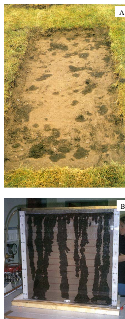
Fig. 8. Fingered flow phenomena in situ and in laboratory experiments. (A) Finger flow in water-repellent sandy soil with permanent grass: 24 h after intensive irrigation the grass layer was removed. Water infiltrates in fingers leaving large sections dry. (B) Evidence of finger flow in laboratory hele-shaw irrigation experiments on dry water repellent sandy soil.
