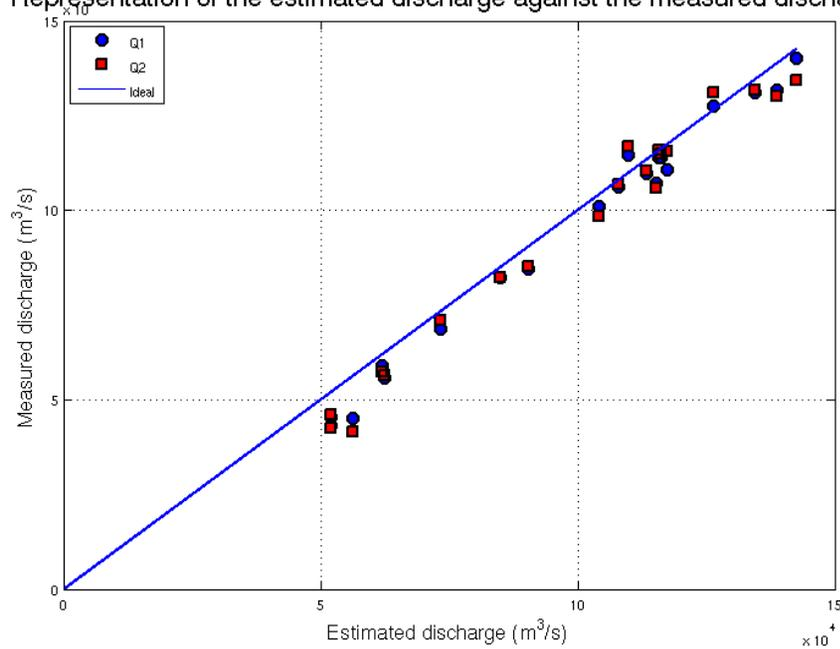
Fig. 1. Comparison of the estimated discharge using Eqs. (8) and (9) and ADCP discharge measurements at Manacapuru gauging station.
