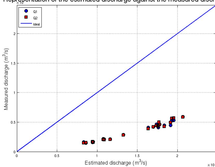
**Fig. 2.** Comparison of the estimated discharge using Eqs. (8) and (9) and ADCP discharge measurements at Obidos gauging station.
