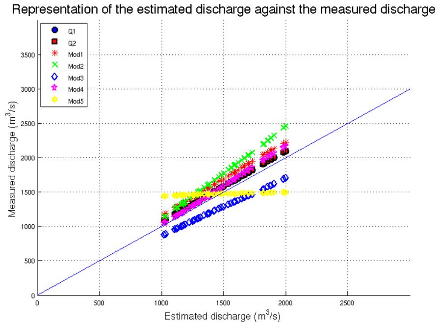
**Fig. 6.** Representation of the estimated discharge against simulated discharge measurements.[Title Page](#)[Abstract](#)[Introduction](#)[Conclusions](#)[References](#)[Tables](#)[Figures](#)[◀](#)[▶](#)[◀](#)[▶](#)[Back](#)[Close](#)[Full Screen / Esc](#)[Printer-friendly Version](#)[Interactive Discussion](#)
