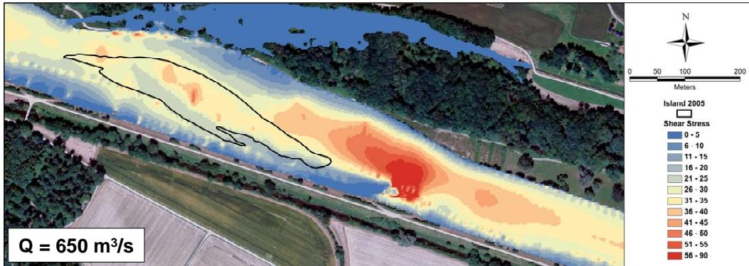
**Fig. 6.** Simulated bed shear stress produced by the maximum flow peak (corresponding to  $650 \text{ m}^3/\text{s}$ ) registered in the range of time 2005–2006. Those kind of simulation have been used to decide the location of Salix plots as well as for morphodynamic analysis. In black it is shown the shoreline of the island for  $30 \text{ m}^3/\text{s}$  (2005).
