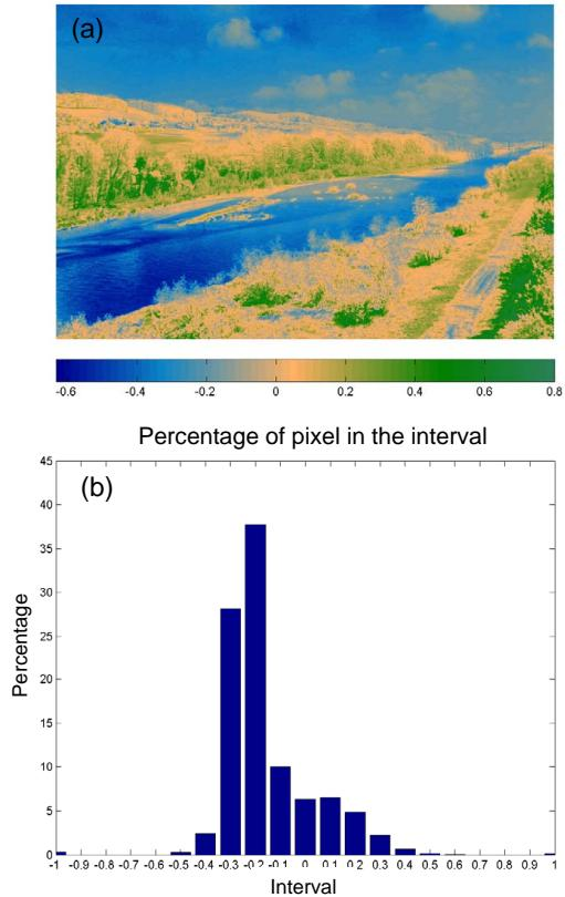
**Fig. 9.** NDVI picture of the field site **(a)** on 3 May 2009. Pixels between 0.1 and 0.8 correspond to vegetation cover, pixels ranging from −0.2 and 0.1 represents bare soil and values smaller than −0.2 water. NDVI images are used to compute the frequency (as a percentage) of vegetation, bare soil and water at a certain time **(b)**.
