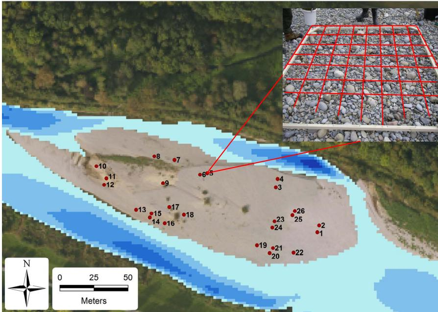
**Fig. 5.** Map of the study island showing the location of vegetation plot in 2009. Plot location is decided according mainly to hydraulic parameters (flow shear stress and velocity) and according to topography (elevation). The upper right corner box shows the matrix frame used for cutting plantation. One cutting is planted in the soil in correspondence of each node. We thus have a regular matrix which helps to identify cuttings position during monitoring.
