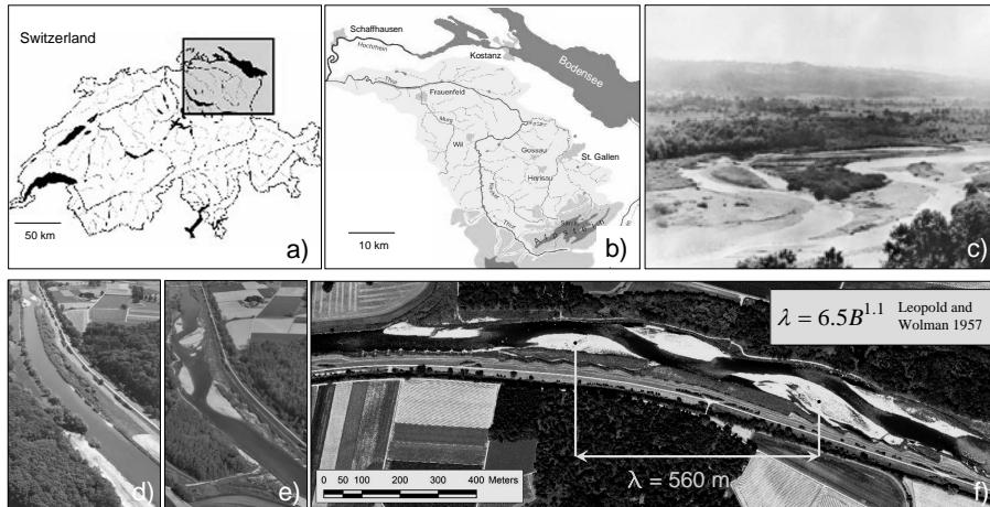
**Fig. 1.** Location of the river Thur in Switzerland (a) and river basin (b). From a natural braiding state (c) the river was straightened (d) in the past century to improve flood protection, to increase agriculture areas and to reduce spreading of disease. As a consequence river bed faced serious erosion problems. After the restoration project started in 2002 the river naturally formed an alternate bar system (e, f).
