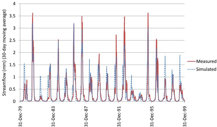
**Fig. 4.** Observed and simulated streamflows in the calibrated GWLF model.
