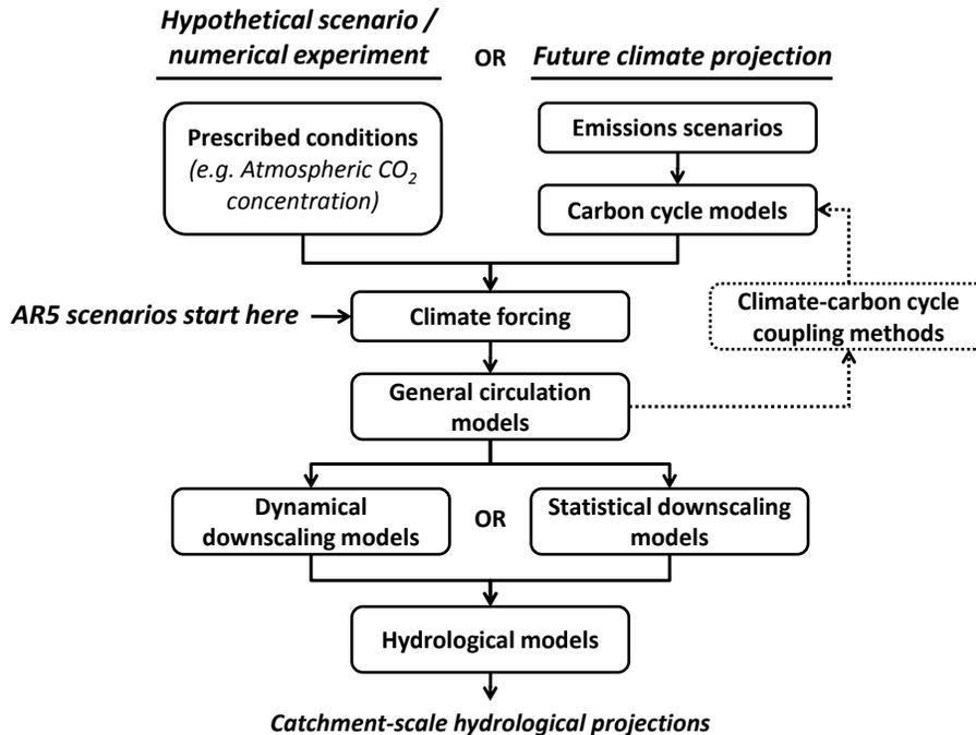
**Fig. 1.** Simplified chart of the main processes involved in modeling hydrological impacts from climate change. Note: dashed lines around climate-carbon cycle coupling methods indicate that not all models are coupled.
