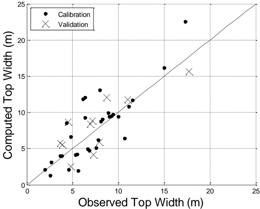
**Fig. 8.** Observed versus computed top width values for the calibration and validation datasets. The 1 : 1 line is shown.
