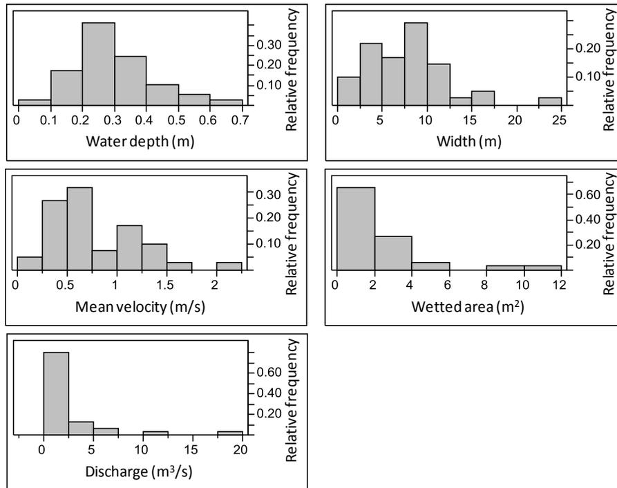
**Fig. 5.** Distribution of the AFIG hydraulic characteristics.
