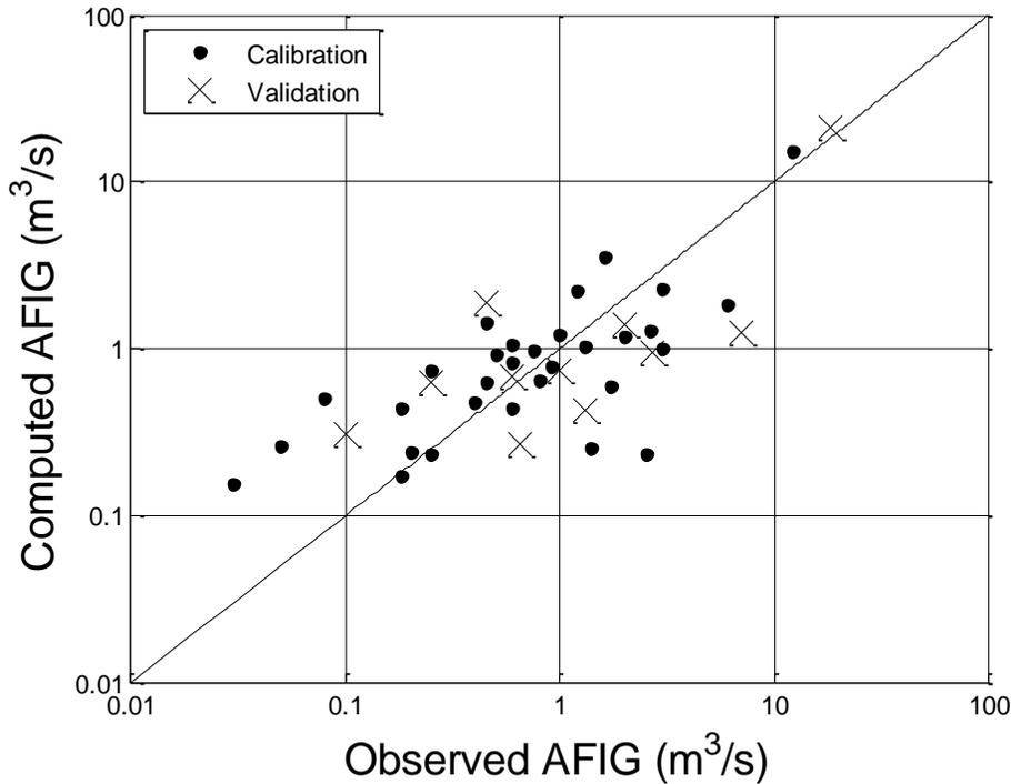
**Fig. 7.** Observed versus computed discharge values for the calibration and validation datasets (note the final equations presented in Table 4 were derived from the full data set). The 1 : 1 line is shown.
