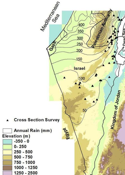
**Fig. 1.** A topographic map with the location of the surveyed cross sections. Annual climatic isohyets are also indicated.
