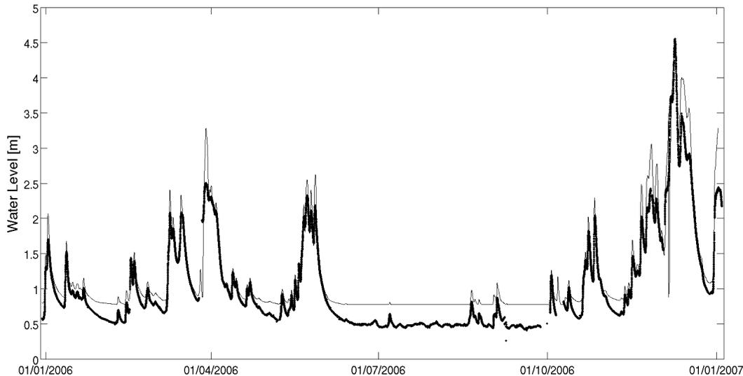
**Fig. 2.** Summary plots of the data available for Welshbridge during the calibration period. Points represent observed data with the line being the concatenation of the output of the most recent hydraulic model initialisation. A bias in the prediction of low flows is clearly shown as are periods of missing data and poor model initialisation.
