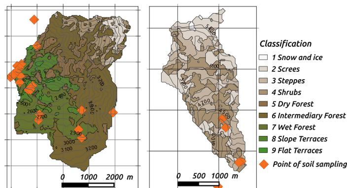
**Figure 4.** Classification of surfaces defined for the two Kharikhola and Tauche subcatchments, established using the supervised classification tool of the QGIS Semi-Automatic Classification Plugin (Congedo 2015), based on Sentinel2 images at a 10-m resolution (Drusch *et al.* 2012). In situ sample points were used to describe the soil and vegetation characteristics of each class.
