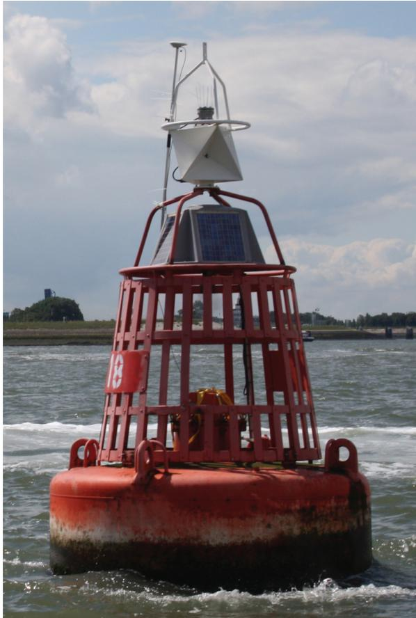
**Fig. 2.** Buoy 18 in the Westerscheldt is located near the town of Terneuzen. On this buoy a Trimble R7 GPS receiver is mounted inside the cage. The Trimble Zephyr (survey) antenna is installed on a range pole on top of the buoy. Note the eddies induced by the tidal current around the buoy.
