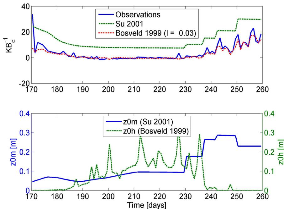
**Fig. 5.** Top panel: Seasonal variation in the daily  $kB^{-1}$  values for the maize canopy, calculated from observations, the parameterizations from Su (2001) and Bosveld et al. (1999). In the bottom panel the roughness length for heat and momentum is shown for Su (2001) and for the new  $kB^{-1}$  parameterization. The new values of the roughness length for heat, are calculated using the  $kB^{-1}$  parameterization of Bosveld (1999), and the roughness length for momentum by Su (2001).
