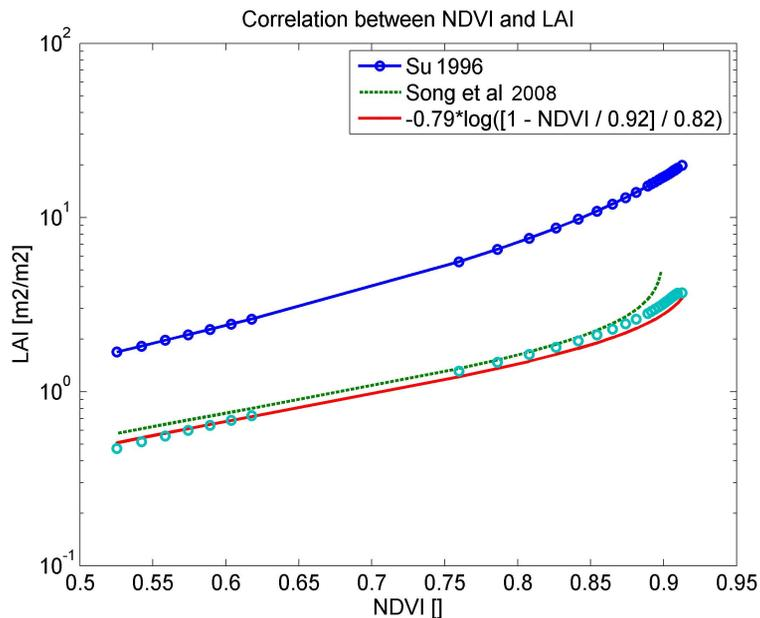
**Fig. 3.** NDVI – LAI relationships. The LAI values obtained by measurements (open circles) and the Su (line with closed circles) and Song parameterizations are shown. The Song parameterization is shown with its original values (the green dotted) for A and B and also for the optimized values (solid red line).
