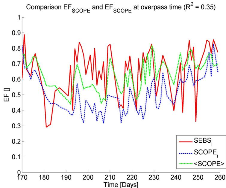
**Fig. 8.** Variation in evaporative fraction during the maize growing season. Evaporative fractions at overpass time calculated by SEBS and SCOPE are shown, as well as the daily average values of the evaporative fraction by SCOPE.
