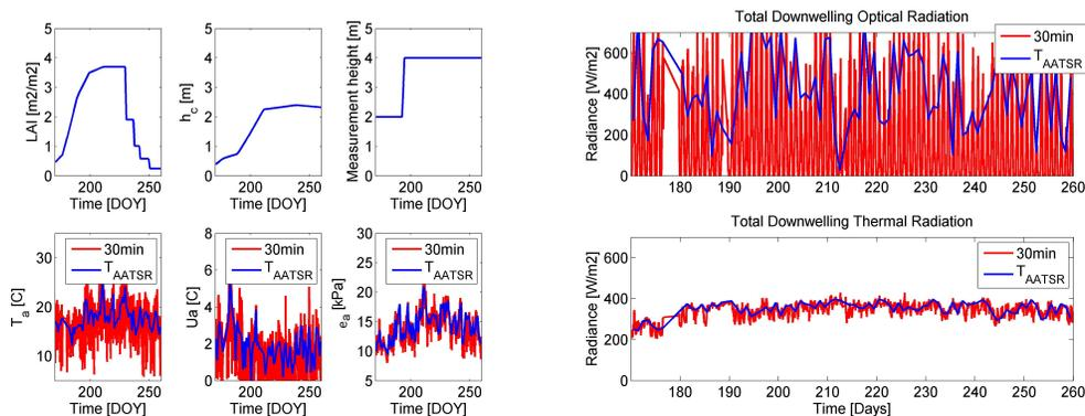
**Fig. 2.** SCOPE input parameters and variables measured at the experimental site during 2002. In the top left panel the surface parameters are shown. In the bottom left panel the atmospheric driving variables. In the right panel the incoming optical and thermal radiance data are shown. The red lines depict half hourly in situ measured data, and the blue lines depict the values at AATSR overpass time ( $T_{\text{aatsr}}$ ).
