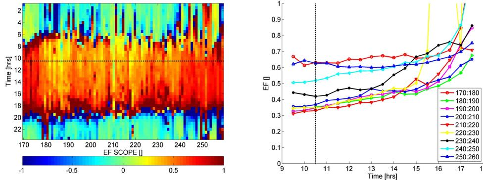
**Fig. 7.** Diurnal variation of the evaporative fraction during the maize growing season. In the left panel the diurnal evaporative fraction as calculated by the SCOPE model for each separate day is shown. In the right panel the 10-day average of the diurnal evaporative fraction as calculated with SCOPE is shown. The dotted line represents the overpass time of AATSR.
