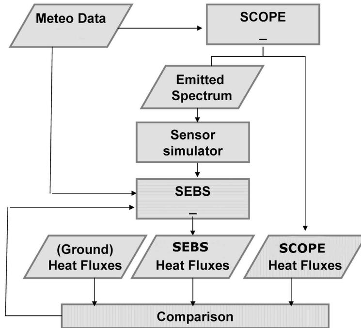
**Fig. 1.** Methodology flowchart for comparing SEBS with SCOPE.
