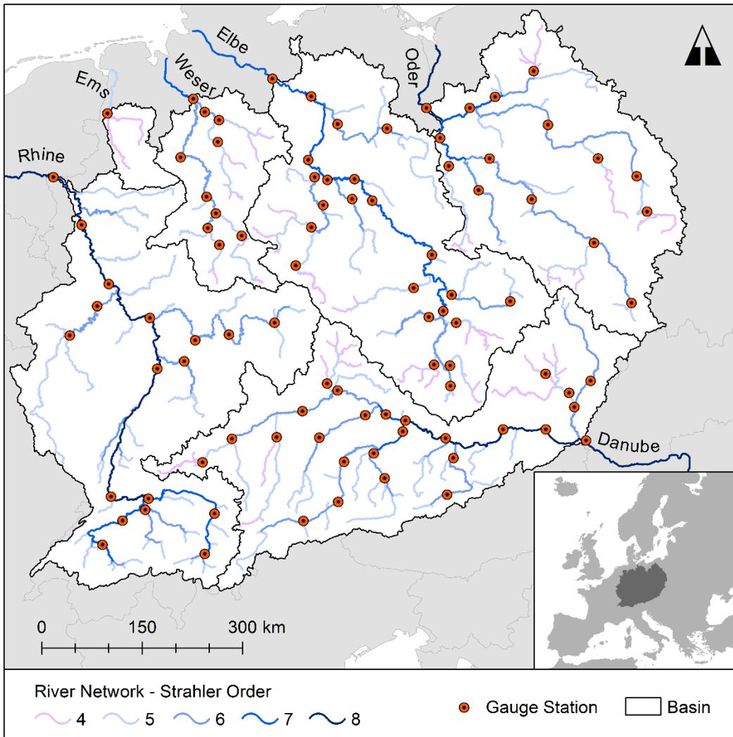
Figure 1: Gauge stations in the area of interest. **Their subcatchments are Strahler stream order is distinguished by color.**
