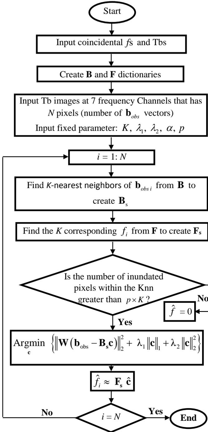
Figure 3. Flowchart of the inundation retrieval algorithm for  $N$  pixels in each orbit. See text for definitions of the notations and detailed explanation.
