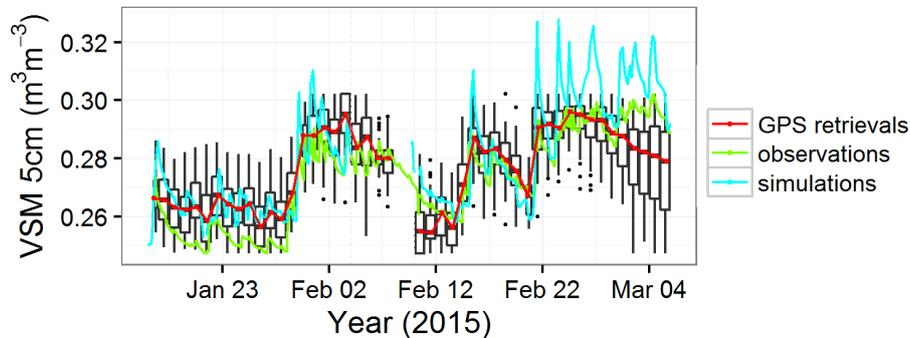
**Figure R2.4** - In situ daily mean surface volumetric soil moisture (VSM) observations at 5 cm depth (green line), ISBA daily mean simulations (blue line), median of the daily GPS retrievals with soil wetness index (red line) and their daily statistical distribution (black box plots) for all available satellite tracks from 16 January to 5 March 2015.
