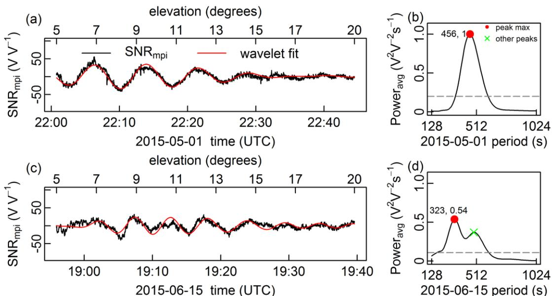
**Figure R2.11** - Examples of (a) usable and (c) unusable track data sets from the ascending tracks of GPS01 on 1 May 2015 and 15 June 2015, respectively: (a, c) multipath SNR data, and (b, d) average power spectrums. The red lines in (a, c) are the reconstructed SNR data by the daughter wavelet corresponding to the maximum peak periods in (b, d), respectively. The green crosses in (d) shows there is more than one peak in the track data, indicating poor quality, unusable data.
