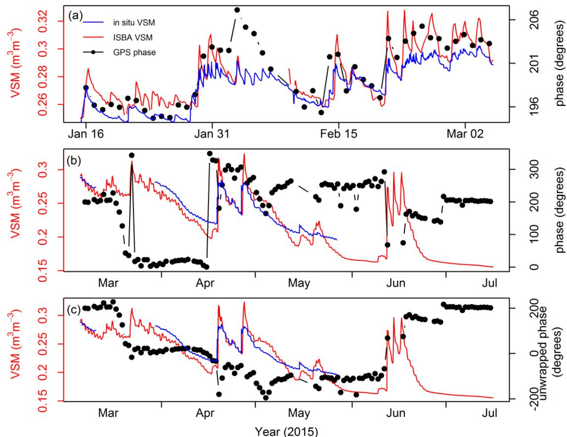
**Figure R2.8** - Example of a track data set (descending tracks from GPS10): (a) from 16 January to 5 March, with no significant vegetation effects; (b) and (c) from 6 March to 15 July, with significant vegetation effects. In (a) and (b), multipath phases (black dots) are compared with *in situ* VSM measurements at 5 cm (blue line) and ISBA simulations (red line). In (c), unwrapped multipath phases (black dots) are used to compare with *in situ* and simulated VSM.
