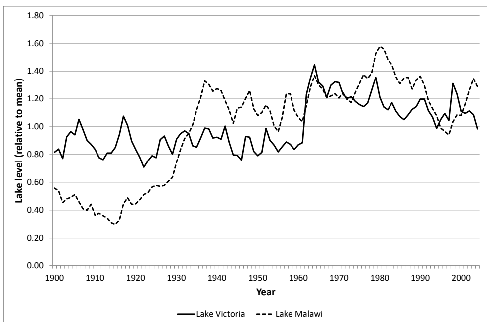
Figure 1. Annual lake level variations in Lake Victoria and Lake Malawi from 1900 to 2004 relative to the mean values in that period; values are expressed in terms of indicative depths at the lake outlet
