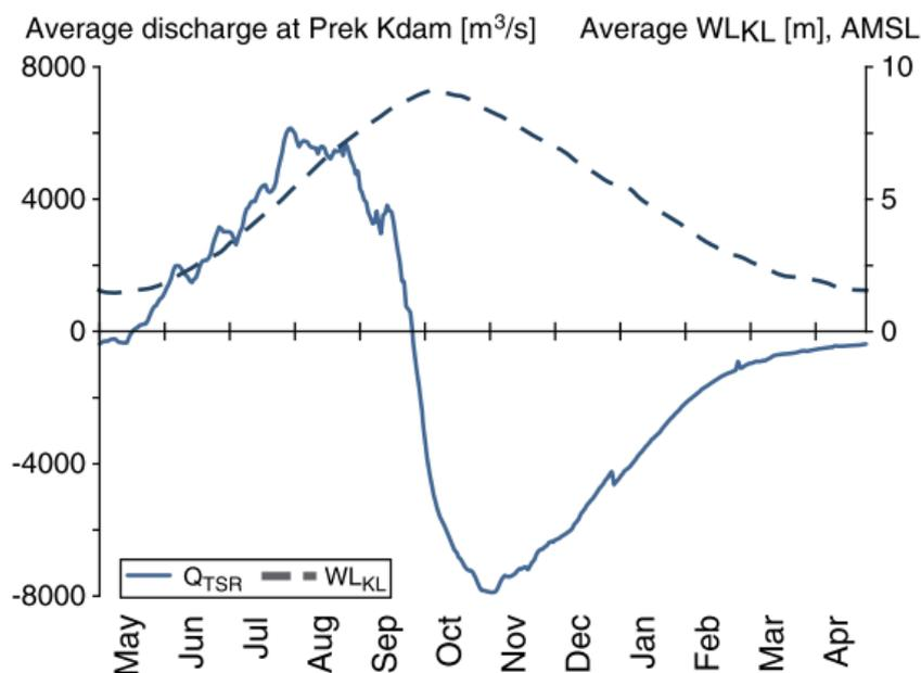
Figure 6. Daily averaged (from 1997 to 2004) water discharge hydrograph at Prek KDam and water level variation at Kampong Luong (Kummu et al., 2014). The solid line presents river flow coming in the Tonle Sap Lake at the Prek KDam station, while the dashed line shows water levels at Kampong Luong station.
